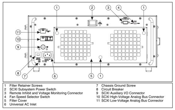
Figure 1-2. Rear View of the PXI-1052 Chassis
